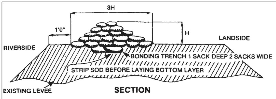
Figure D.5 Sketch of a typical levee raise with bonding trench.
