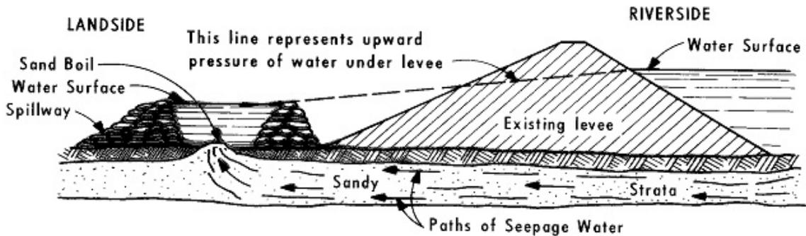
**Figure D.6** To treat the sandboil, the pressure of the seepage water is counterbalanced by hydrostatic pressure from the column of water in the ring levee.
